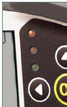
**The three LED lights** on the display unit indicate whether the couplings are within tolerance (green light), within double tolerance (orange light), or out of double tolerance (red).
