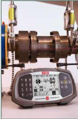
Several of its features are adopted from the innovative Fixturlaser XA system, which will reduce the time spent on pre-alignment actions, measurement registration, performing the actual alignment, remeasuring to make certain that you have a correctly aligned machine; and, finally, documenting the measurement data.
