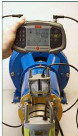
**The measurements can be transferred to a PC** by connecting the display unit to the USB connection. When connected the display unit appears as a mass storage device in your PC. Files are then easily transferred using the Explorer on the PC.
